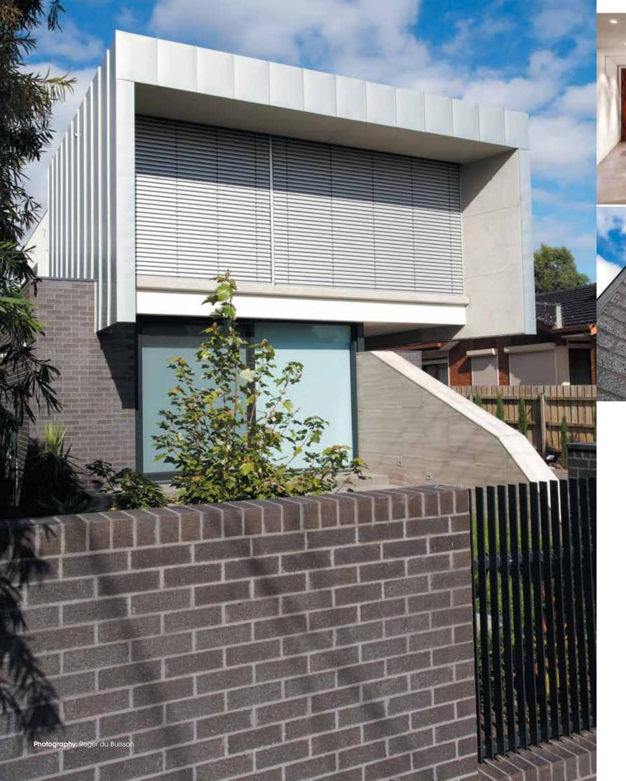
**previous page.** As dusk falls the glaze of the bricks takes on a glow. The brickwork spanning the outdoor room is supported on an L-shaped lintel
